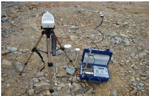
Fig. 1. Vibration monitoring on bedrock.
