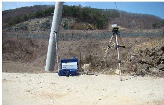
Fig. 3. Vibration monitoring on soil.
