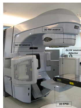
그림 1. The medical linear accelerator with the on-board imager mounted in orthogonal to the megavoltage beam direction
