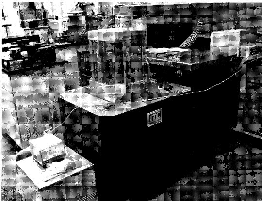
Fig. 4 Interlaken Simple Performance Testing Equipment
