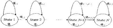
Fig. 4 The state transition model for generating target outputs of a neural network
