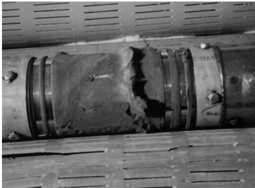
Fig. 2. Broken expansion packer tube.
