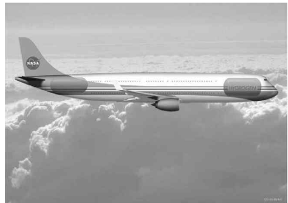
Fig. 2 Hydrogen Transport Aircraft with Hydrogen Tanks in Fuselage
