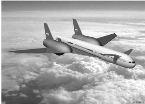
Fig. 3 Conceptual Hydrogen Aircraft with Wing Hydrogen Tanks
