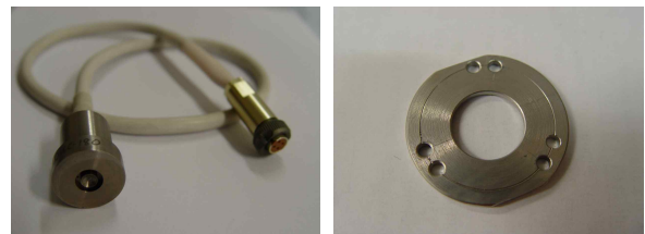
Fig. 3 Loadcell and Fixation Ring
