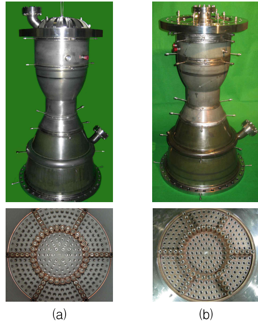
Fig. 1 Photographs of regenerative cooling combustion chambers: (a) CC#1 and (b) CC#2
