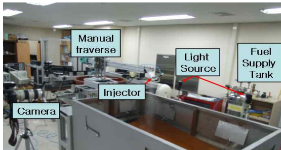
Fig. 2 Spray visualization test rig
