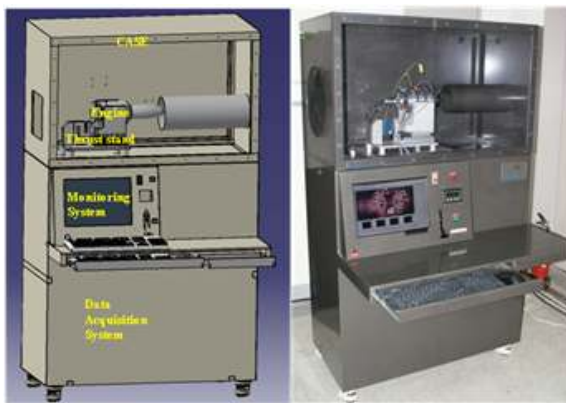
Fig. 2 Complete Test Setup of I-jet 130
