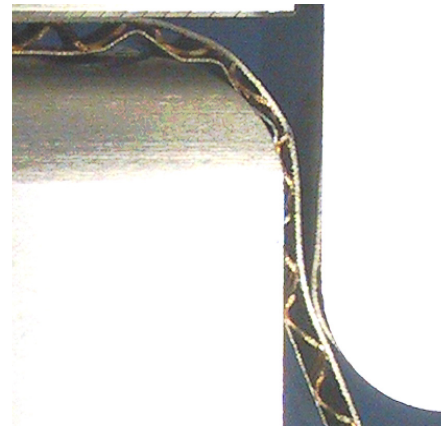
Figure 3. Deformation of sandwich sheet according to the location of bend line (clearance=3.3 mm) at stroke of (a) 0 mm, (b) 15 mm and (c) 30 mm.
