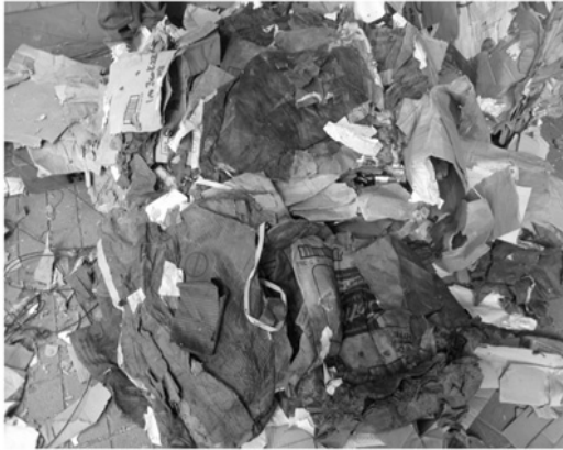
Fig. 3. Water soaked portions in core side of bale.
