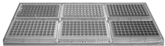
Fig. 8. Pulp mold with 72 holes.
