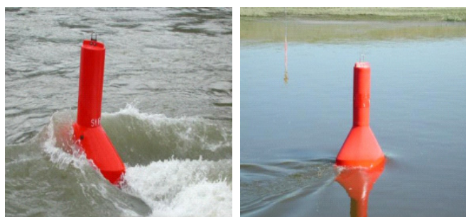
Oval buoy B5 1,0 m/s Oval buoy B7 3,0 m/s
