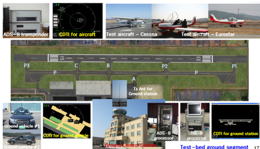
Figure 4 Configuration of the ADS-B test-bed
