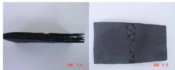
Fig. 9. Photos of carbon fiber composite decomposed in supercritical ethanol
