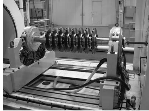
Fig. 1 HDS recycle-gas 8-stages compressor installed using its 5-pads LBP tilting-pad bearings for operating-speed balancing
