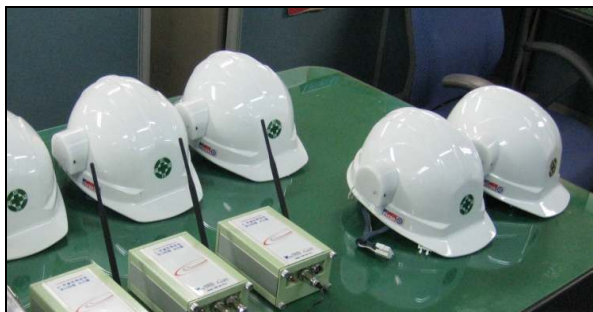
Fig. 2 The pictures of safety helmet attached sensor node and router & sink node
