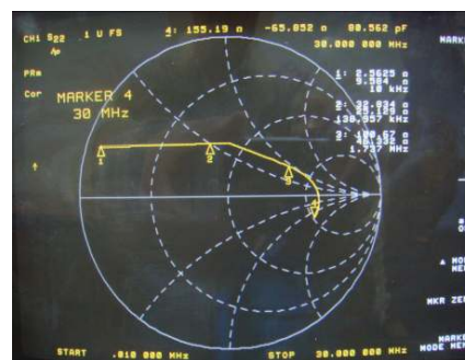
Fig. 4 Test Test results of S-parameter (S11) of unmatched Coupler
