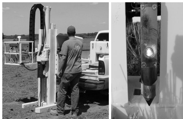
Fig. 3 (a) Soil profile measurement with a probe unit. Fig. 3 (b) A conical probe tip.
