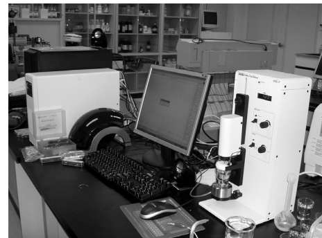
Fig. 1 RDE cell stand consisting of three electrodes (left) and voltammetric analyzer system (right, reproduced from ref. Kim et al. (2008)).
