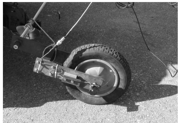
Fig. 4 5th wheel for measuring the real travel distance.
