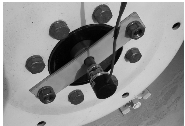
Fig. 3 Device for measuring the theoretical travel distance.
