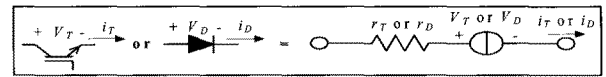
Fig. 3 Equivalent circuit of IGBT or FWD for calculating the conduction loss, where V_T is voltage drop of IGBT; V_D is forward voltage drop of FWD; r_T and r_D are on-state resistances of IGBT and free-wheel diode respectively
