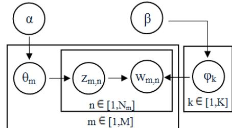
**Fig. 3** An LDA generative graphical model
