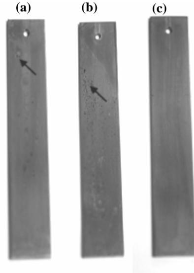
**Fig. 3** The image of each specimen after application of VCI materials and anti-tarnishing solution : (a) No. 5; (b) No. 6; (c) No. 7
