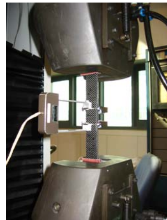
Fig. 7 Installed specimen for tensile test
