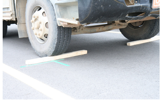
Fig. 11 Impact loading using vehicles
