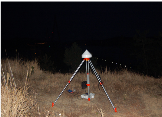
Fig. 4 Reference station of the DGPS system
