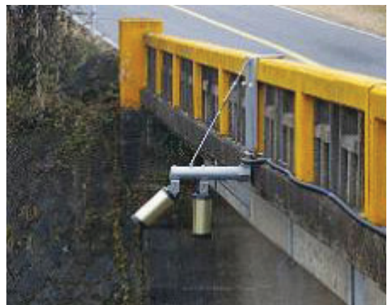
그림 2. The Location(Left; blue solid rectangle) and the state of installation(Right) of stream discharge monitoring equipment at the upstream of Hancheon watershed.
