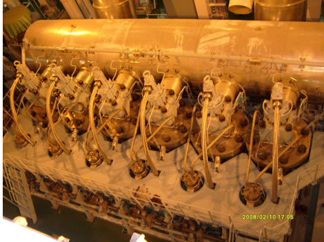
Figure 12: 6S90MC-C engine for power measurement
