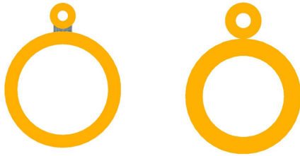
(a) Soldered type (b) Taped type Figure 2 Cross-section of the two SLHX
