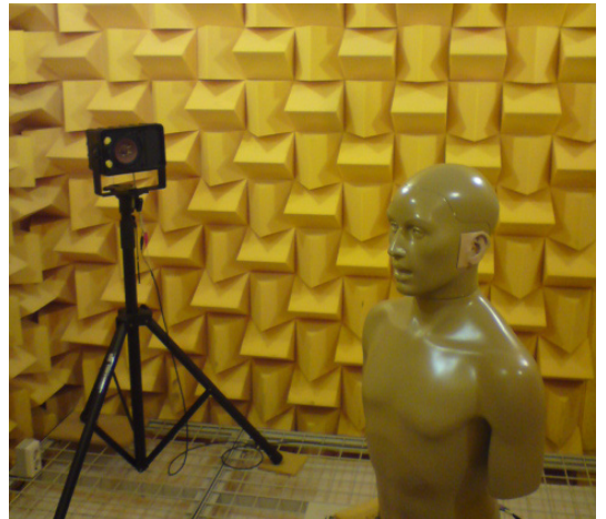
Fig. 3 Experimental set-up for HRTF measurement
