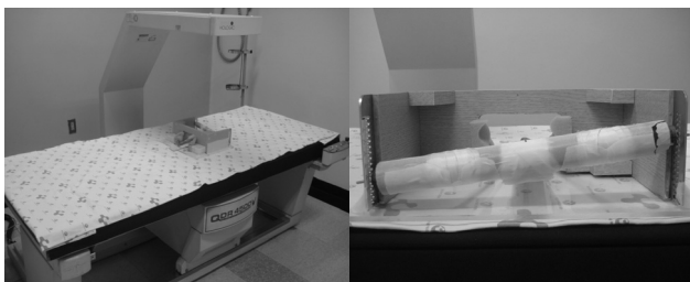
Figure 8. A apparatus for the measurement of BMD of dried cadaver (radius). 4A. A thick acryl plate connected with the middle portion of a rod and both side wooden chopsticks connected with the rod and acryl plate for horizontal balance. 4B. The bottom of a radius closely placed on the acryl plate during the measurement of BMD
