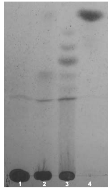
Fig. 5. TLC analysis of galactan reaction products. Of 0.2% (w/v) galactan in 5.0 mM AcB (pH 5.0), 1.0 mL was incubated at 37°C for 2 hr with 4.0 mU GALase (fraction 20, Fig. 3) or 8 hr with 2.0 mU \beta -gal (fraction 10, Fig. 3). The estimated galactan hydrolysis was about 4.0 and 1.0%, respectively. Lane 1, substrate blank (2- or 8-hr incubation); lane 2, galactan incubated with \beta -gal; lane 3, galactan incubated with GALase; and lane 4, galactose (1 g/L).
