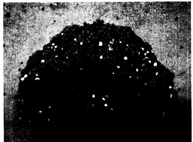
Fig. 5. Mass of fine aggregates stuck together sintered at over 1160°C due to an excess liquid formation.
