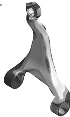
Fig. 6 Initial stress contour for shape optimization
