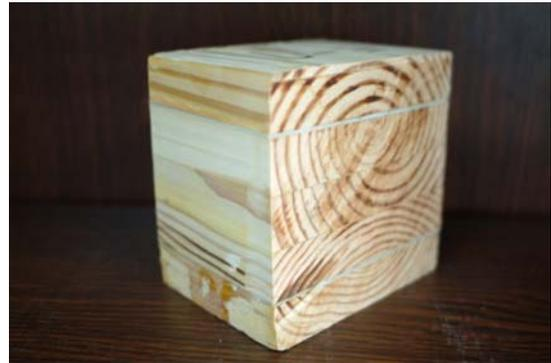
Fig. 3. Shape of delamination test specimen.
