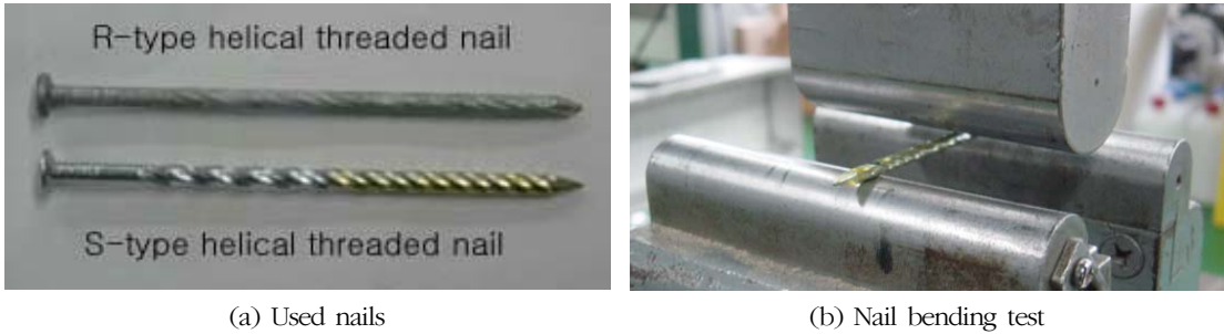
Fig. 1. Used nails and nail bending test.
