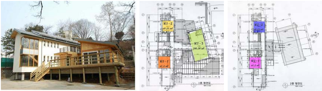
Fig. 1. Test house and places for measuring indoor air quality in a wooden house.
