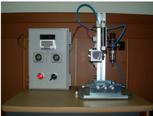
Fig. 2. The device which is designed for the fatigue test
