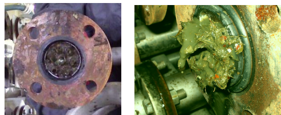
Fig. 9. Clogging at the entrance of the tubular membrane module.
