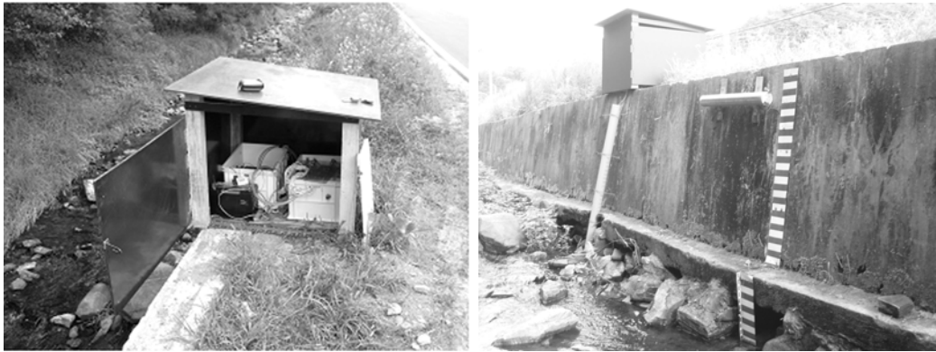
Fig. 4. Flow and automatic water sampler installed at the outlet of Wolgok-ri watershed.
