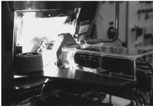
Fig. 3. Sampling from a fluidized-bed reactor and photograph of particle size analyzer equipped with CCD camera (reproduced with permission from T. Tanino and T. Enomoto in Shionogi & Co., LTD.).
