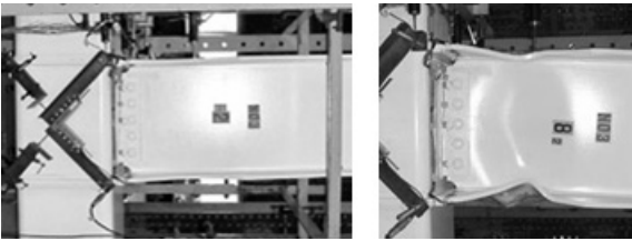
(a) RBS 접합부 실험사례(www.sdr-tech.co.jp)
