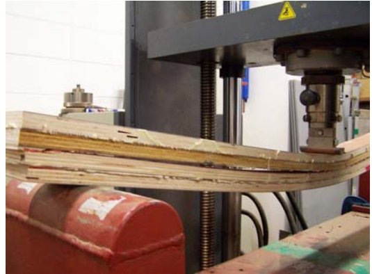
Fig. 5. Failure type of static bending for 4-laminated plywood lumber specimen.
