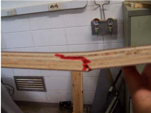
Fig. 4. Failure type of static bending for plywood waste specimen.
