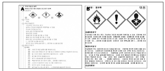
Figure 4. Preparation of labels through MSDS Editing program A : Layout for selecting labelling elements B : The GHS label prepared by MSDS Editing program
