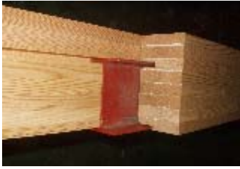
Fig. 1. Composite material beam (Steel H-Glued laminated timber).
