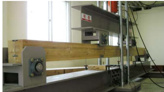
Fig. 7. Bending test of composite material beam on three point loading.
