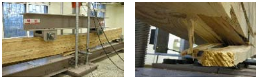
Fig. 10. Breaking shape of glued laminated timber beam II.
