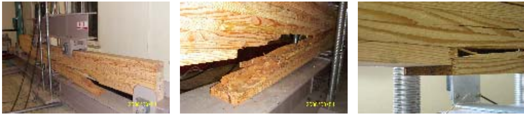
Fig. 9. Breaking shape of glued laminated timber beam I (Finger-joint).
