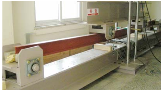
Fig. 6. Bending test of structural steel H beam on three point loading.
