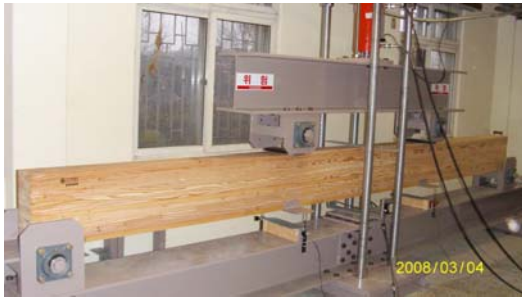
Fig. 5. Bending test of glued laminated timber beam on three point loading.
