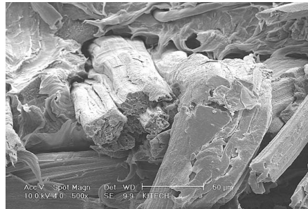
Fig. 14. SEM micrographs of PP/5% NaOH treated kenaf fiber (70/30) interface on composite :50 \mu\text{m} (at 500 \times ).
