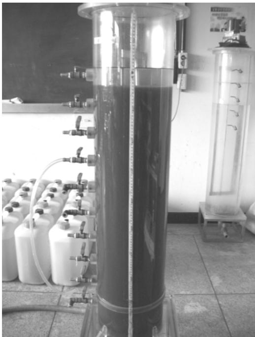
Fig. 1. Settling column for zone settling rate test.
