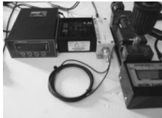
Fig. 5. Digital indicator for measuring compressive force.
