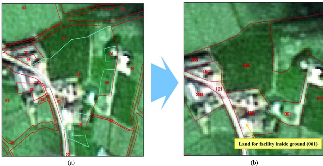
Fig. 6. Classification of forestry-related land cover using land registration document and SPOT-5 Satellite Imagery. (a) land registration document, (b) SPOT-5 Satellite Imagery
